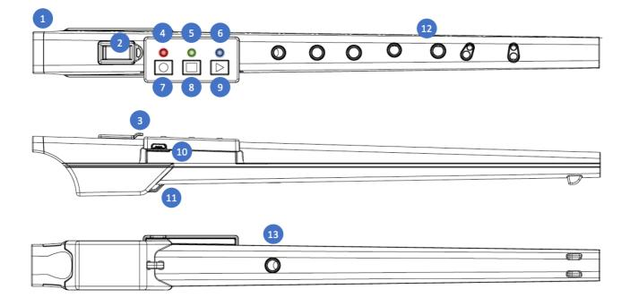
1 Mouthpiece, windway and lip sensor: The mouthpiece, also called embouchure, allows the player to breath into the instrument, generating notes and giving expression to the sound. The windway shapes the air flow to focus on the labium edge. The re.corder electronics detect the presence of your lips to allow continuous calibration and enabling its output. Inside
