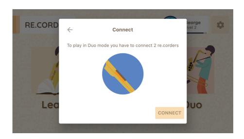
After pressing the 'CONNECT' button you will see the codename of your friend's re.corder on the list, connect with it exactly with the same procedure of your instrument: Press the ROUND button while clicking the name of the recorder, then release the ROUND button when the BLUE led stays ON.
